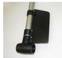
Flow probe prop housing with optional alignment fin
